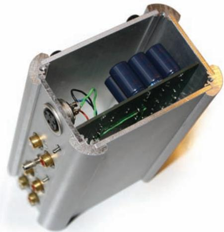
Compact in size and sturdily built, Profono sports a cleverly designed all-aluminium case, with individual corner extrusions holding the aluminium panels together, ensuring a tight, rigid and reliable construction that is quick and efficient to manufacture. Casework of such quality is rare at this price point and serves to protect the internal components, reject sonically deleterious RFI and keep the unit solidly in position when heavy cables are connected.
